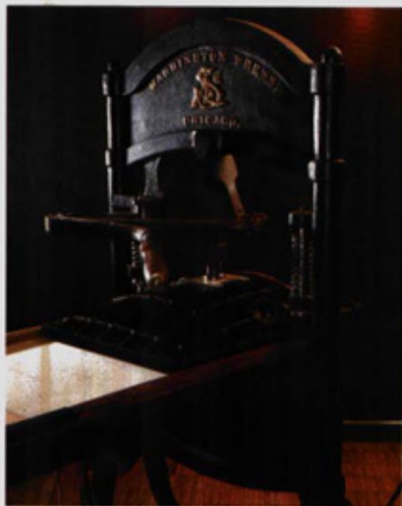
PROOF IT: Stauffer-Flint Hall's 19th-century hand press, destined for Spencer Research Library, was designed to "pull proofs," allowing printers and editors to proofread a job before it was sent to a mechanized press to be printed in large quantities.
