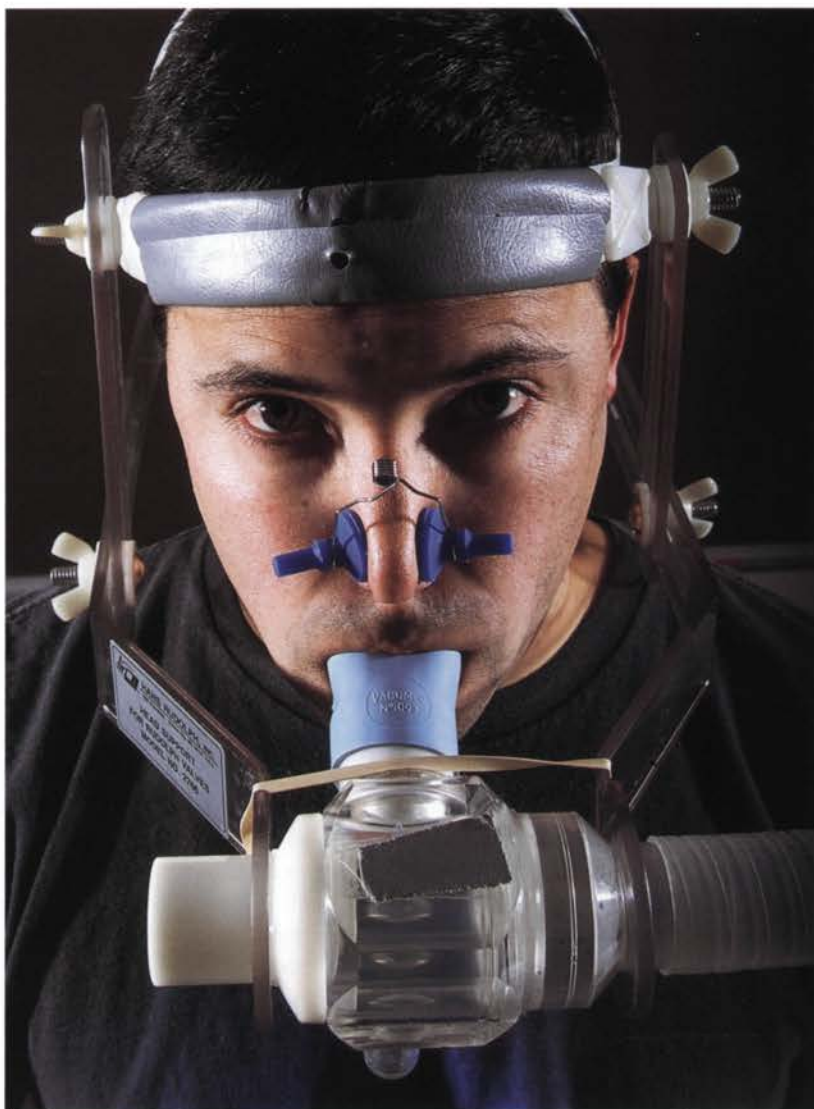
Senior Natalie Skola (p. 20) bikes to VO 2 max in the lab's environmental chamber. The breathing valve (also modeled by doctoral student Jess Acosta, above) connects to a metabolic measurement cart, which gauges cardiorespiratory fitness.
